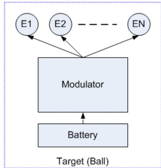
Fig. 5. Infrared Ball Block Diagram
