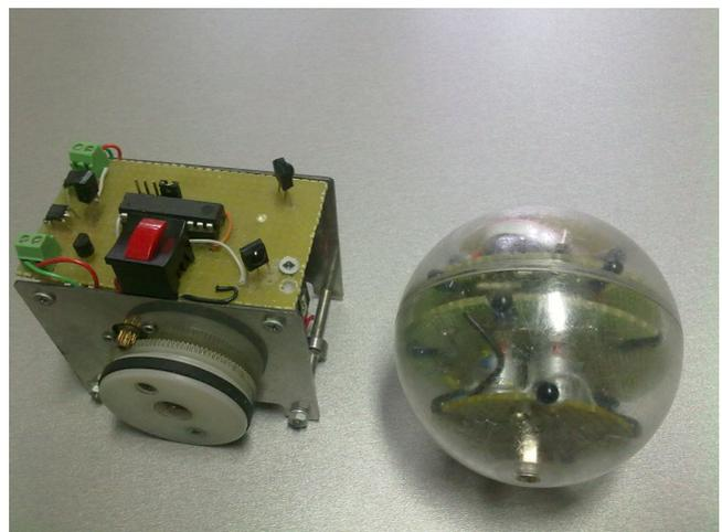
Fig. 1. Infrared Ball Chasing Robot
